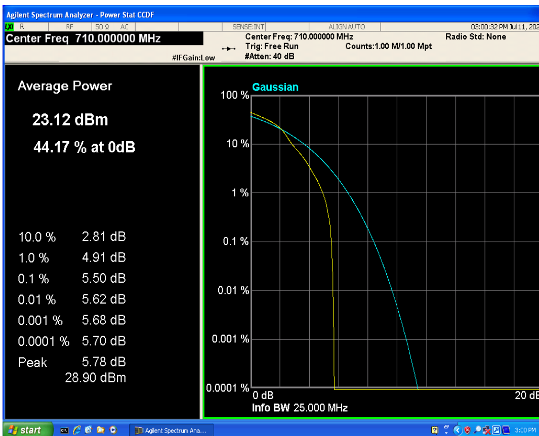
Band17 QAM16 BW=10MHz Channel=23790 RB Size=1 Position=#0
