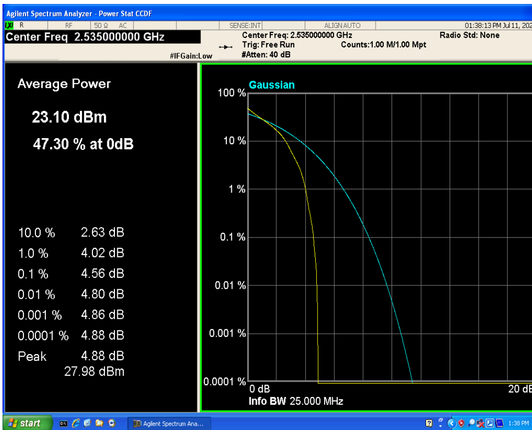
Band7 QAM16 BW=5MHz Channel=21100 RB Size=1 Position=#0
