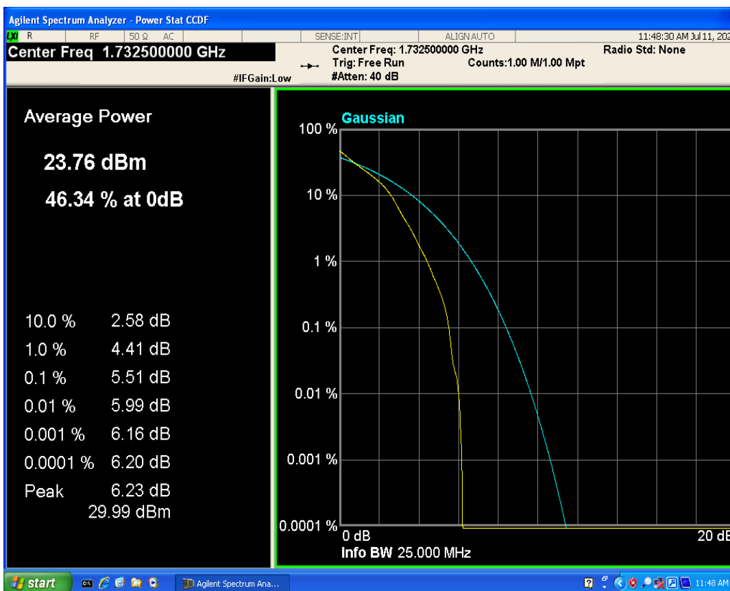
Band4 QAM16 BW=10MHz Channel=20175 RB Size=1 Position=#0
