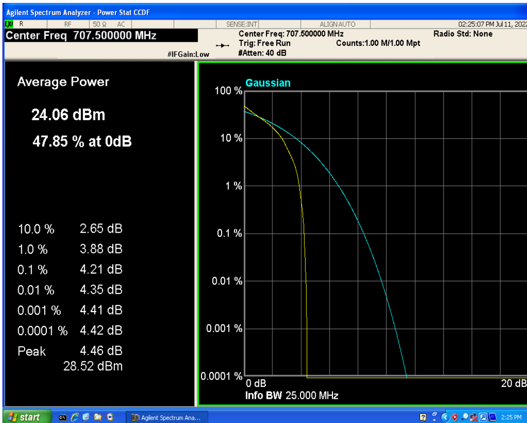
Band12 QAM16 BW=5MHz Channel=23095 RB Size=1 Position=#0
