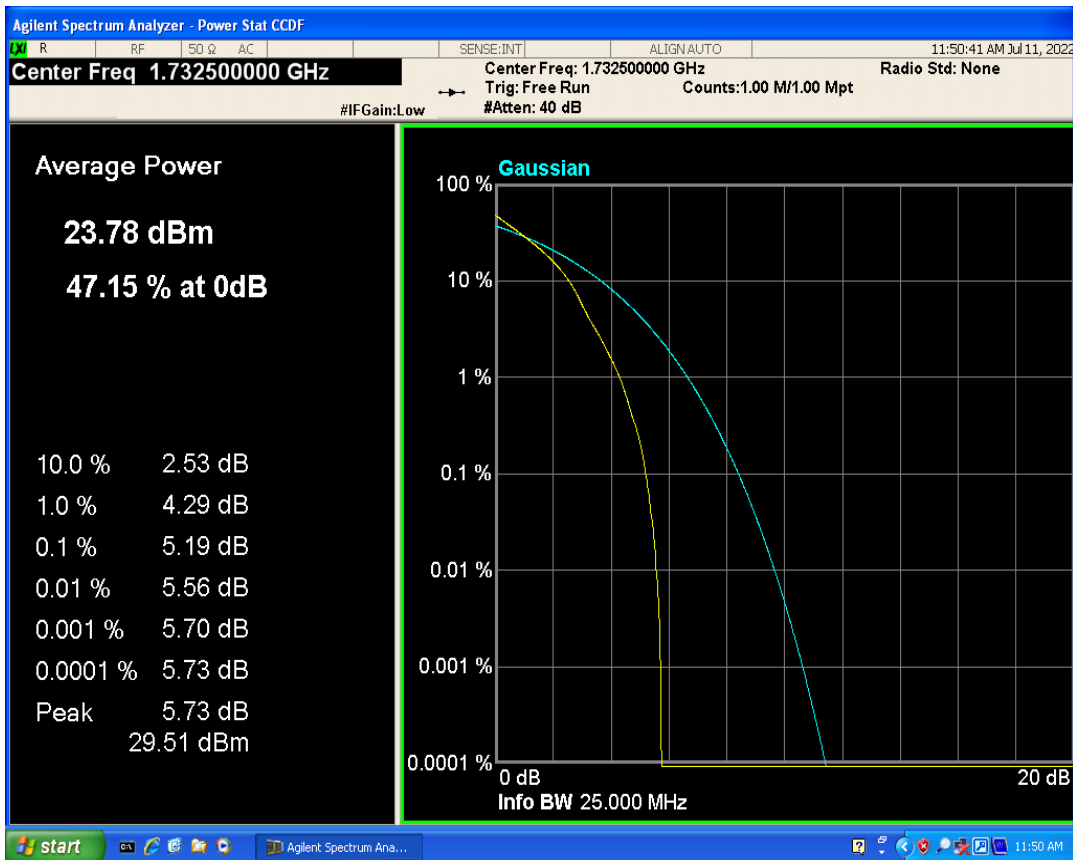
Band4 QAM16 BW=15MHz Channel=20175 RB Size=1 Position=#0
