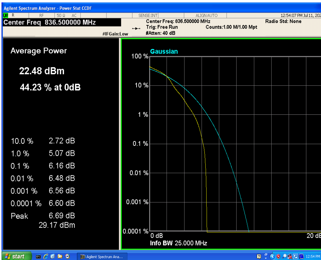
Band7 QPSK BW=5MHz Channel=21100 RB Size=1 Position=#0
