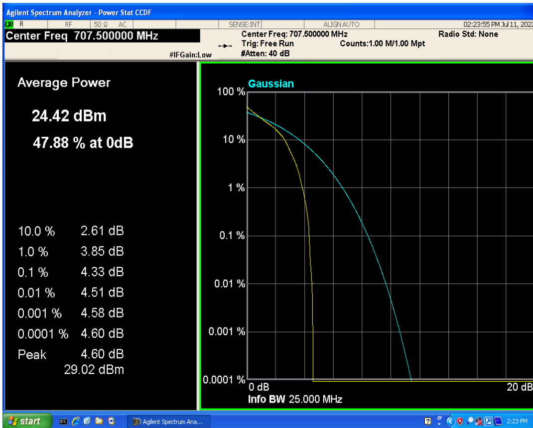
Band12 QAM16 BW=3MHz Channel=23095 RB Size=1 Position=#0
