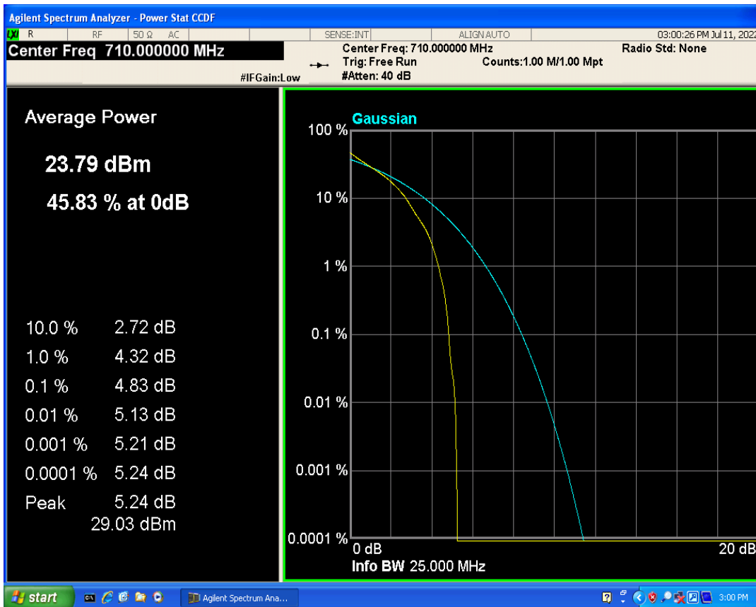
Band17 QPSK BW=10MHz Channel=23790 RB Size=1 Position=#0
