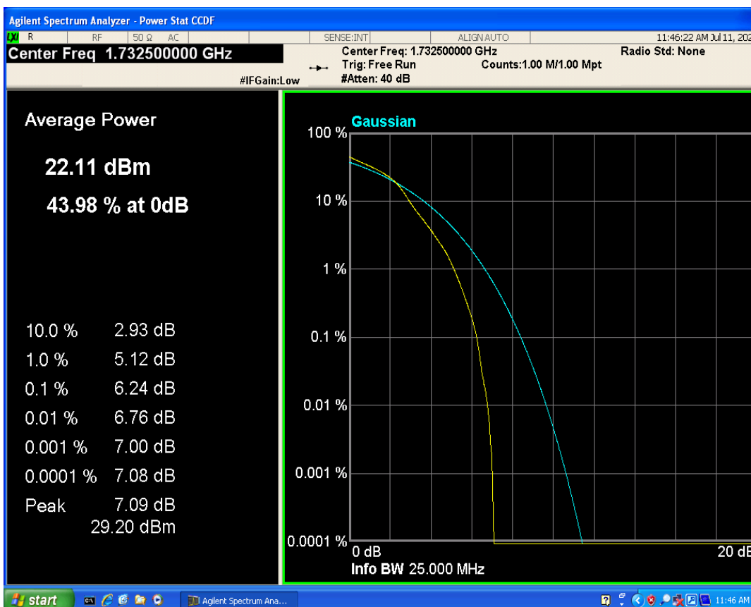
Band4 QPSK BW=10MHz Channel=20175 RB Size=1 Position=#0
