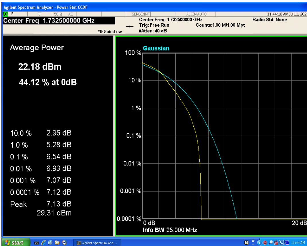
Band4 QAM16 BW=5MHz Channel=20175 RB Size=1 Position=#0
