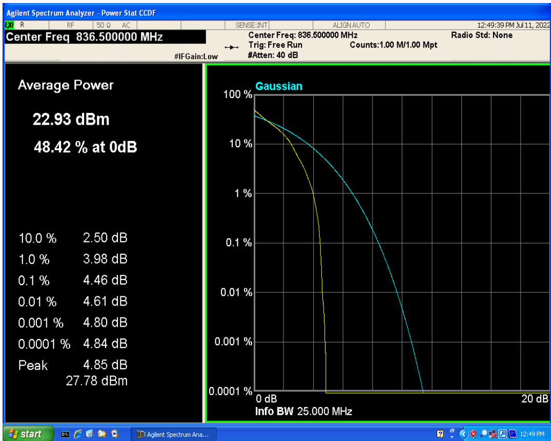
Band5 QPSK BW=5MHz Channel=20525 RB Size=1 Position=#0
