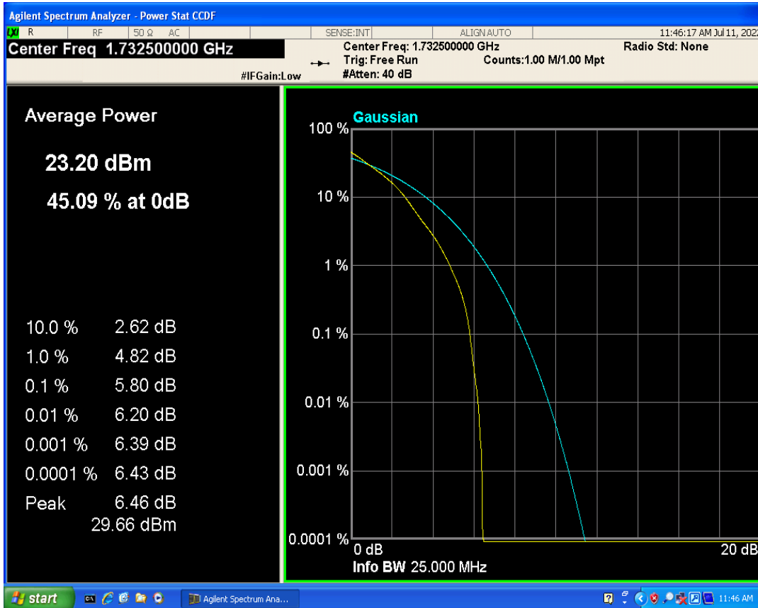
Band4 QAM16 BW=3MHz Channel=20175 RB Size=1 Position=#0
