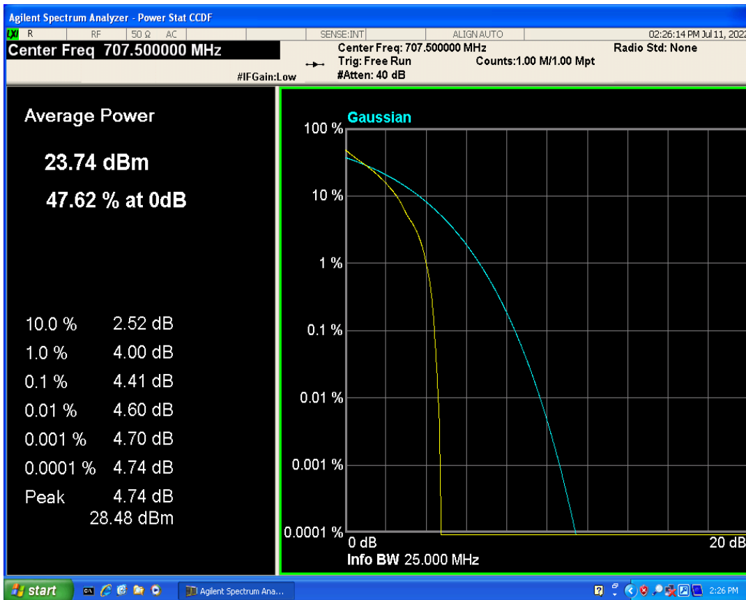
Band12 QAM16 BW=10MHz Channel=23095 RB Size=1 Position=#0
