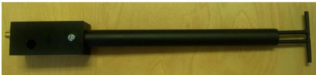
Figure 1 – MVG COMOSAR Validation Dipole
