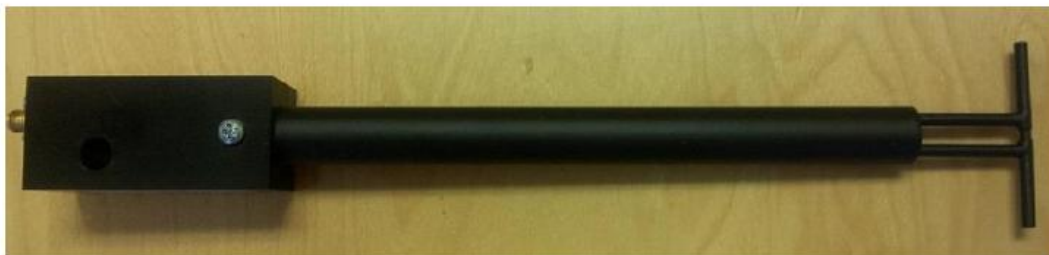
Figure 1 – MVG COMOSAR Validation Dipole
