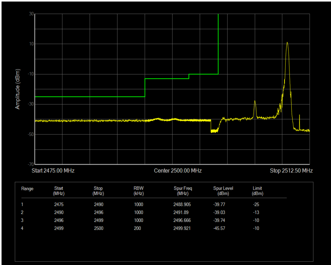
Band7 QPSK BW=10MHz Channel=20800 RB Size=50 Position=#0
