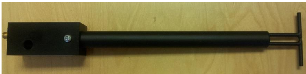
Figure 1 – MVG COMOSAR Validation Dipole
