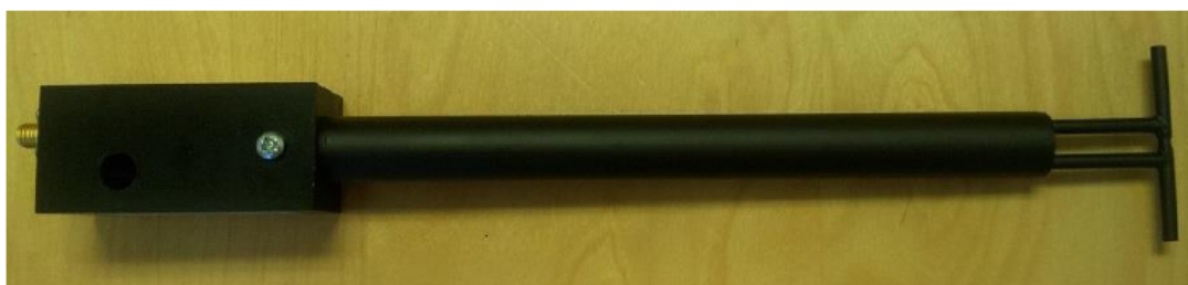
Figure 1 – MVG COMOSAR Validation Dipole
