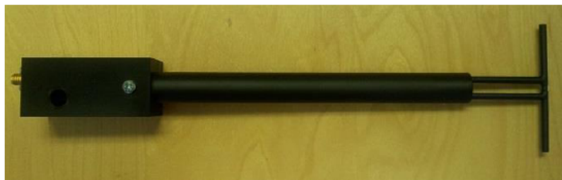
Figure 1 – MVG COMOSAR Validation Dipole
