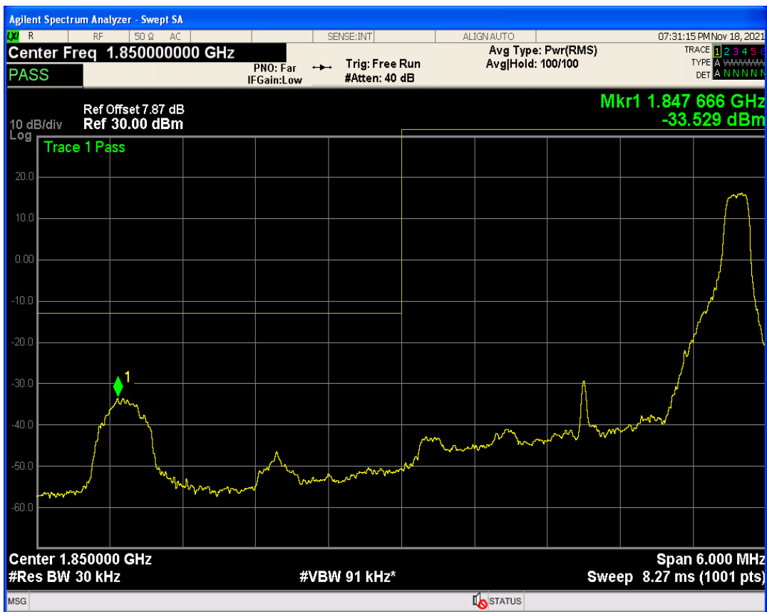
Band2 QAM16 BW=3MHz Channel=18615 RB Size=1 Position=#0
