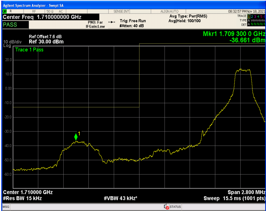
Band4 QAM16 BW=1.4MHz Channel=19957 RB Size=1 Position=#0
