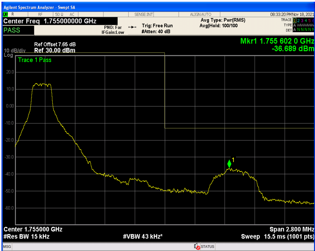
Band4 QPSK BW=1.4MHz Channel=20393 RB Size=1 Position=#Max
