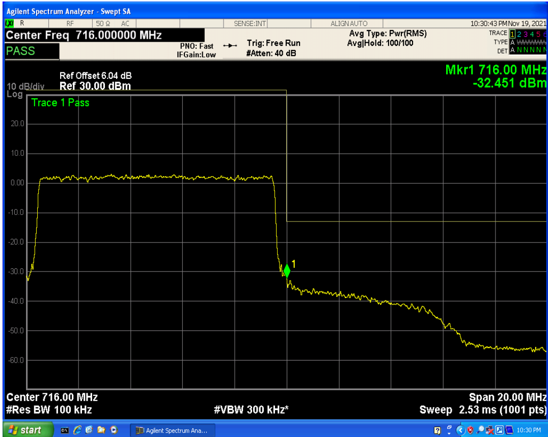
Band2 QPSK BW=1.4MHz Channel=18607 RB Size=1 Position=#0
