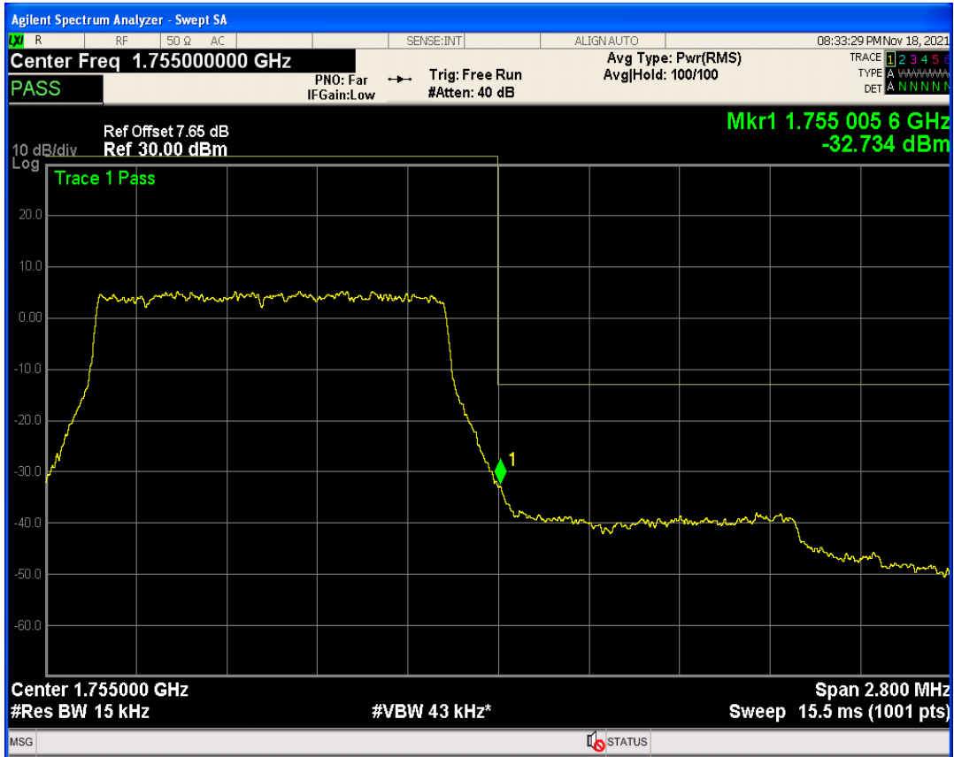
Band4 QAM16 BW=1.4MHz Channel=20393 RB Size=6 Position=#0
