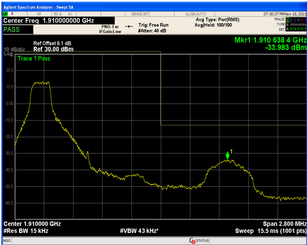
Band2 QPSK BW=1.4MHz Channel=19193 RB Size=1 Position=#Max
