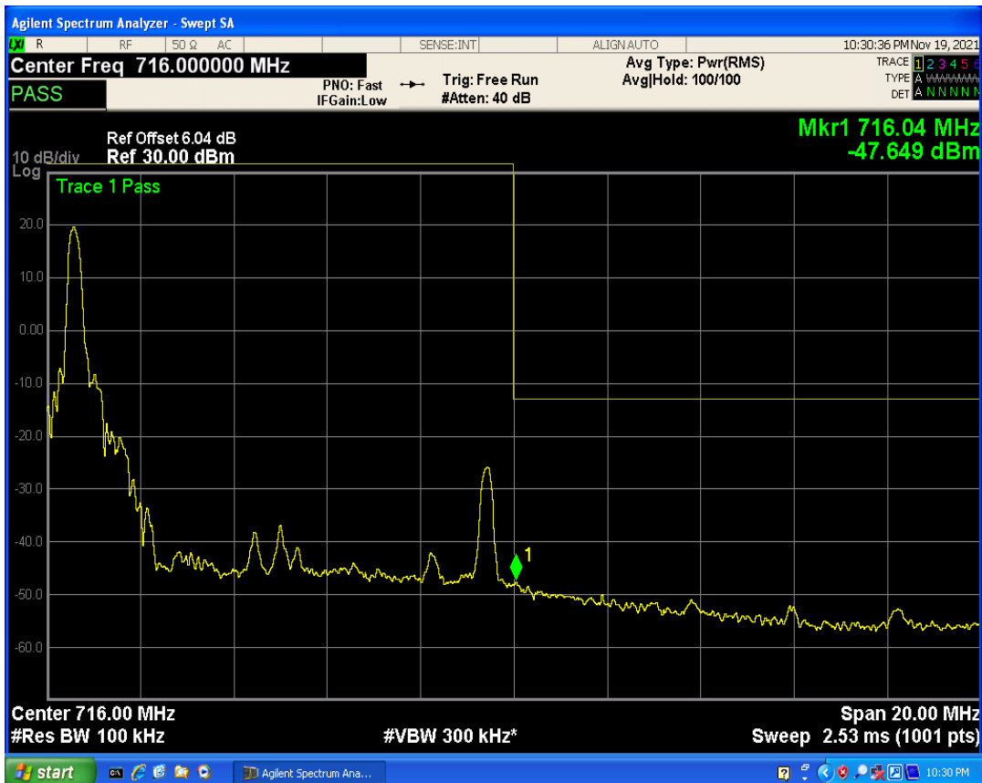
Band17 QPSK BW=10MHz Channel=23800 RB Size=50 Position=#0
