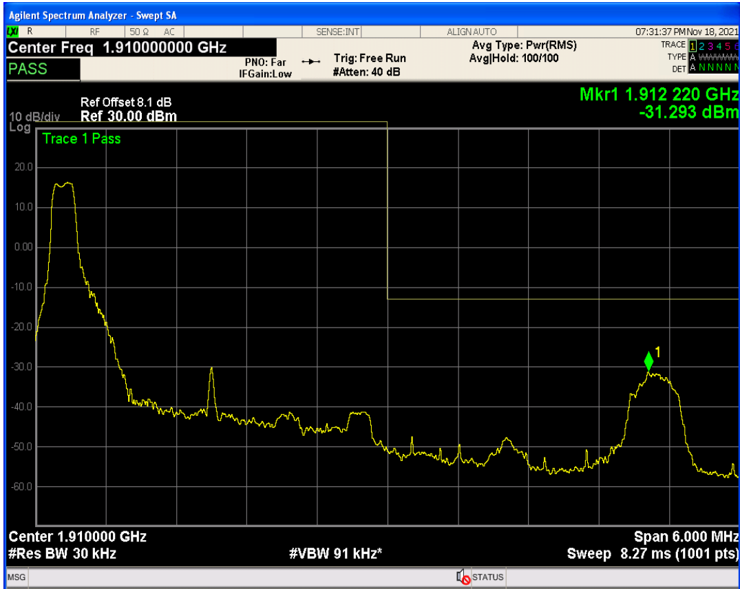
Band2 QPSK BW=3MHz Channel=19185 RB Size=15 Position=#0
