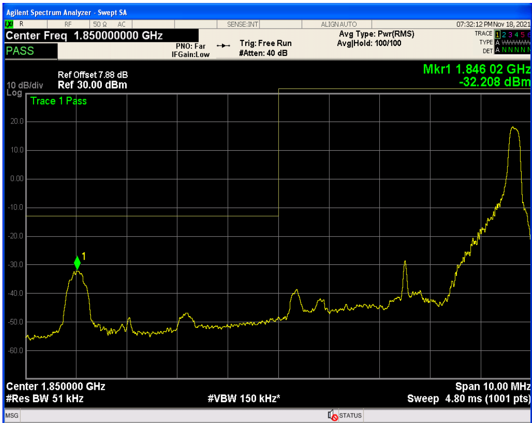
Band2 QPSK BW=5MHz Channel=18625 RB Size=1 Position=#0
