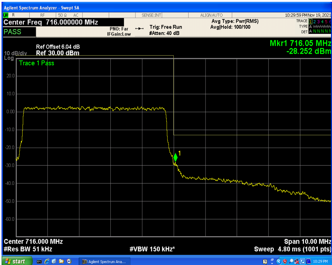
Band17 QPSK BW=10MHz Channel=23780 RB Size=1 Position=#Max
