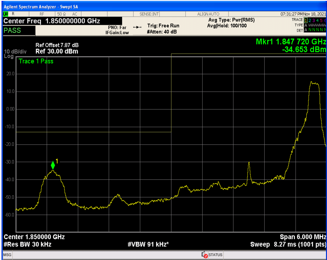
Band2 QPSK BW=3MHz Channel=19185 RB Size=1 Position=#Max
