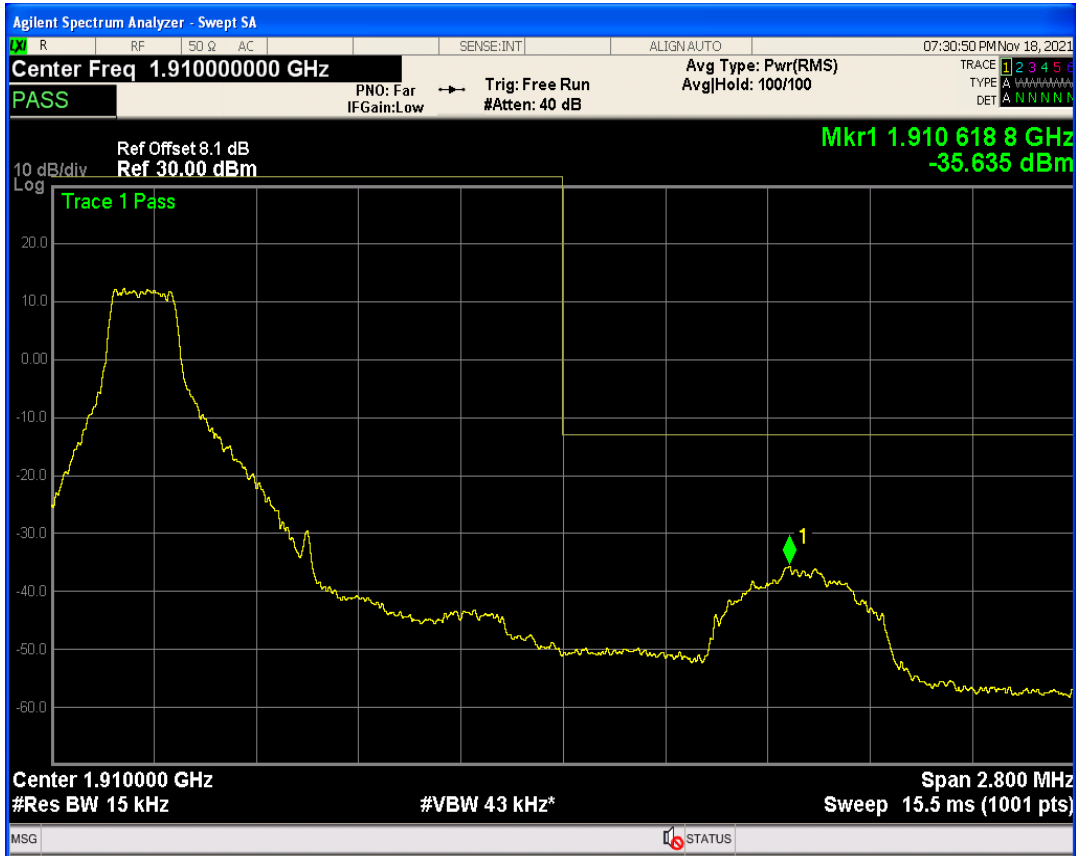
Band2 QAM16 BW=1.4MHz Channel=19193 RB Size=6 Position=#0
