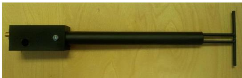
Figure 1 – MVG COMOSAR Validation Dipole
