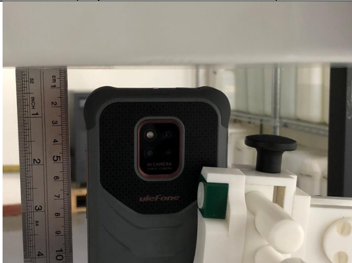
Top Side (Separation distance of 10mm)
