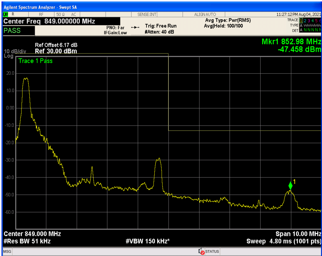
Band5 QAM16 BW=5MHz Channel=20625 RB Size=1 Position=#0
