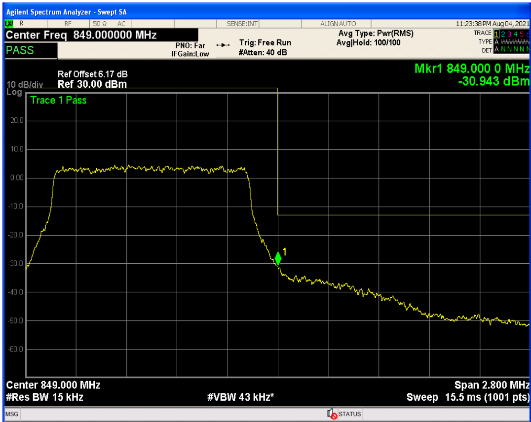
Band5 QPSK BW=3MHz Channel=20415 RB Size=1 Position=#0
