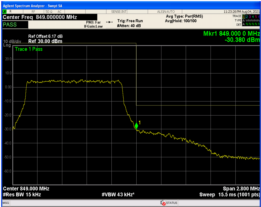
Band5 QPSK BW=1.4MHz Channel=20643 RB Size=6 Position=#0
