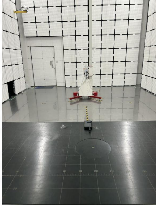
Transmitter unwanted emissions in the spurious domain (30MHz to 1GHz) Receiver spurious emissions (30MHz to 1GHz)
