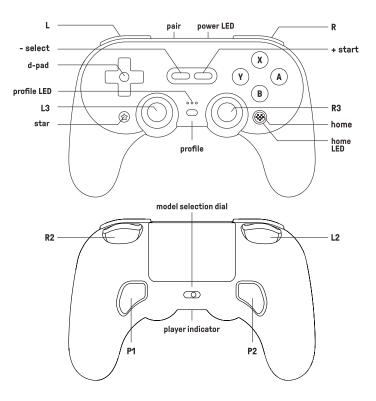
press & hold start for 3 seconds to turn off the controller press start to turn on the controlle
