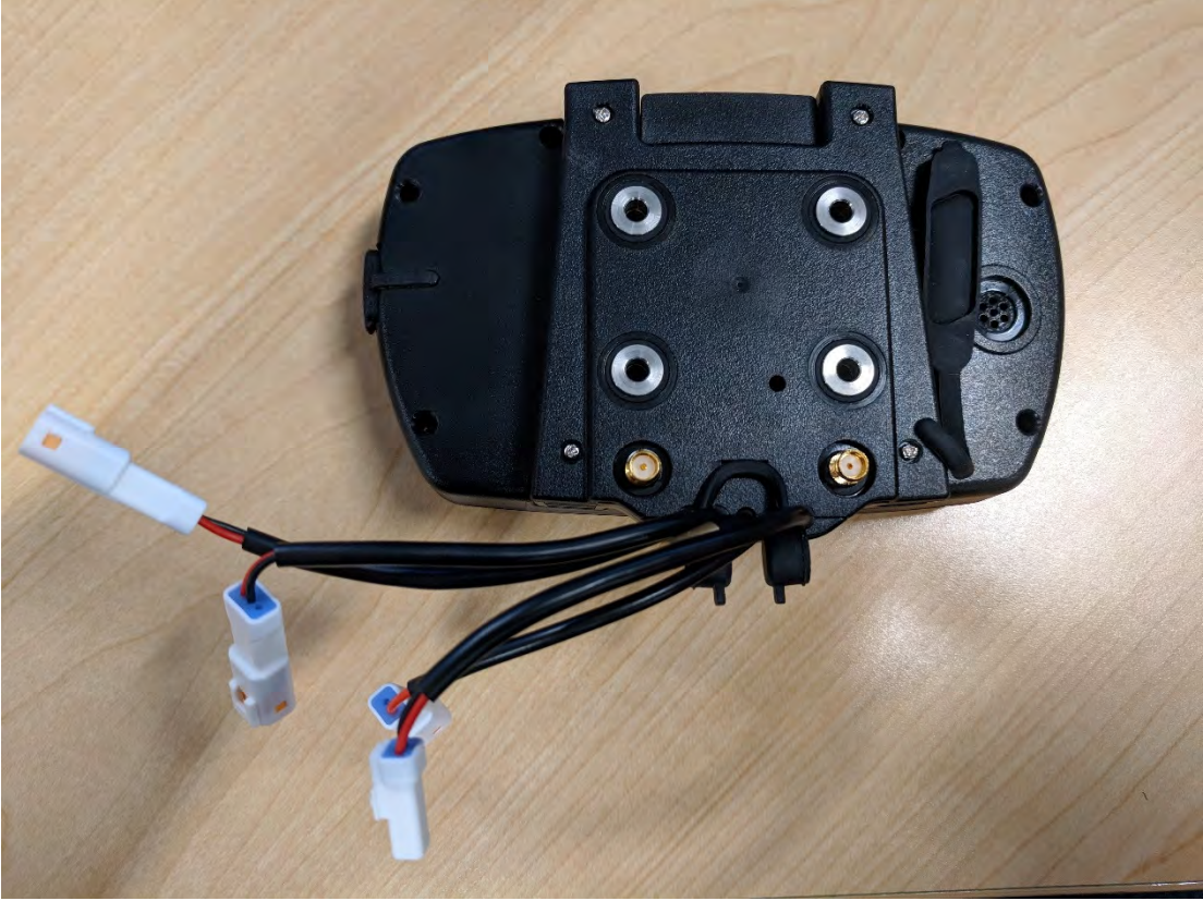
Bracket as it appears when attached to the main unit, with antenna connectors visible
