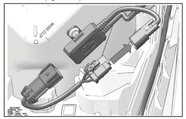
6. Install cable ties ② around wiring.
