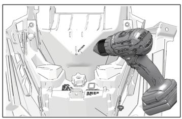
3. Install controller using push-pin rivet 4.
