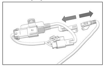
2. Disconnect grill lights adapter pigtail from module.
