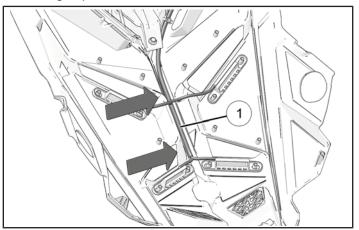
6. Install kept grill inserts on mounting standoffs. Make sure grill insert accent light ① wiring is placed under grill inserts.
