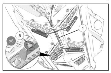
8. Attach grill inserts using eight clips ⑤. Make sure grill insert accent light ① wiring is not pinched.
