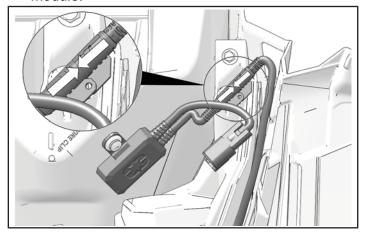
5. Connect pigtail adapter to module.
