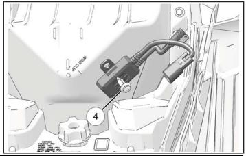
4. Connect grill insert accent light lead to control module.
