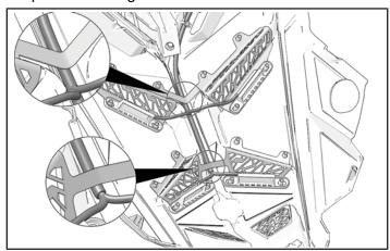
7. Install grill insert accent light ① onto grill standoffs using eight clips ⑤. Install lights on front side of grill openings.
