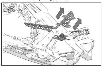
5. Put grill insert accent lights ① on hood. Make sure wiring is placed in center rib on hood.
