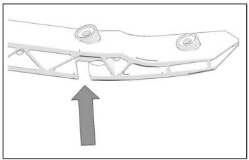
5. Attach handguard accent light using two kept screws. Tighten until fully-seated.
