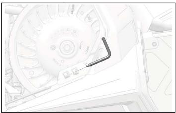
8. Install two push pin rivets.
