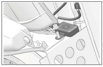
12. Remove plug from chassis connector. Connect harness
