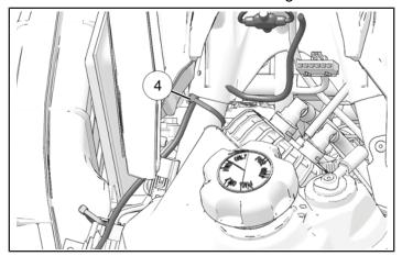
15. Attach wiring to steering post using cable ties 4.
