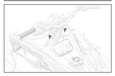
6. Install two screws and one push pin rivet. Torque screws to specification.
