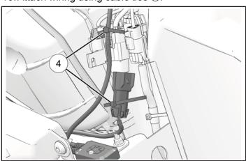
14. Attach harness to chassis tube using cable tie 4.
