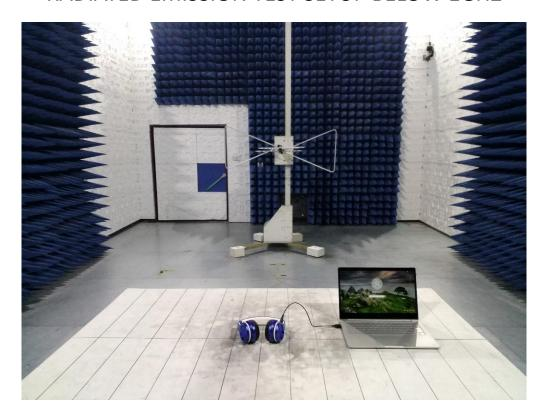
RADIATED EMISSION TEST SETUP ABOVE 1GHZ
