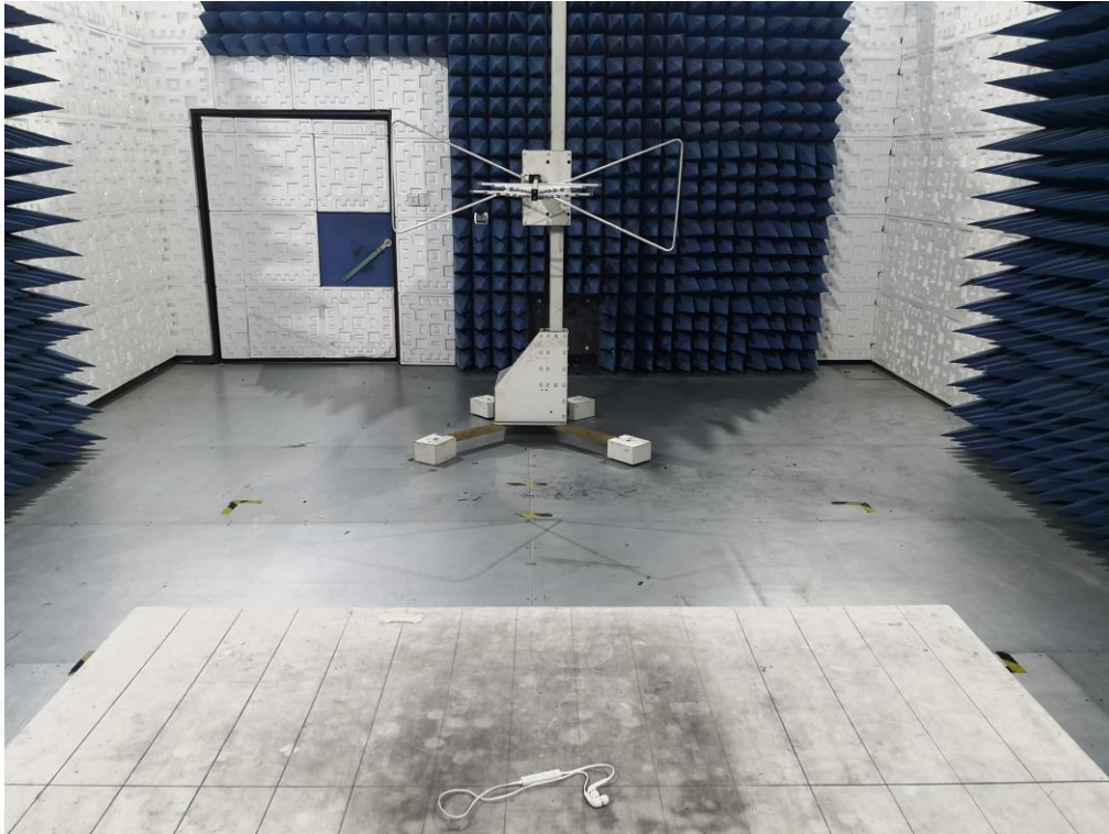
RADIATED EMISSION TEST SETUP ABOVE 1GHZ
