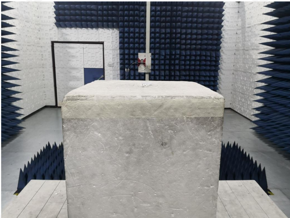
RADIATED EMISSION TEST SETUP ABOVE 1GHZ
