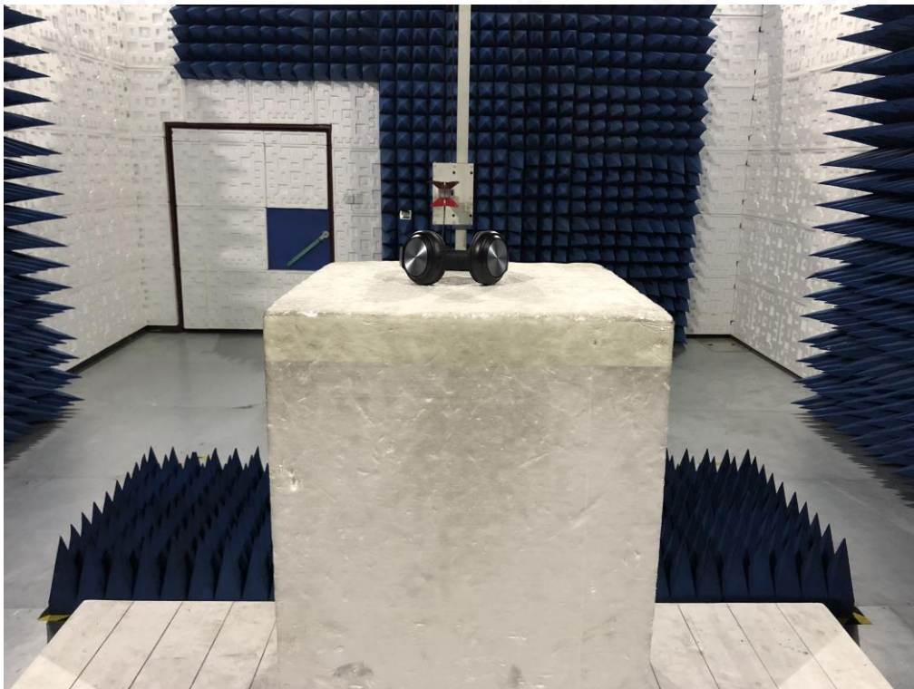
RADIATED EMISSION TEST SETUP ABOVE 1GHZ
