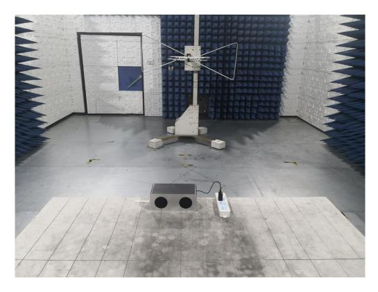
RADIATED EMISSION TEST SETUP ABOVE 1GHZ
