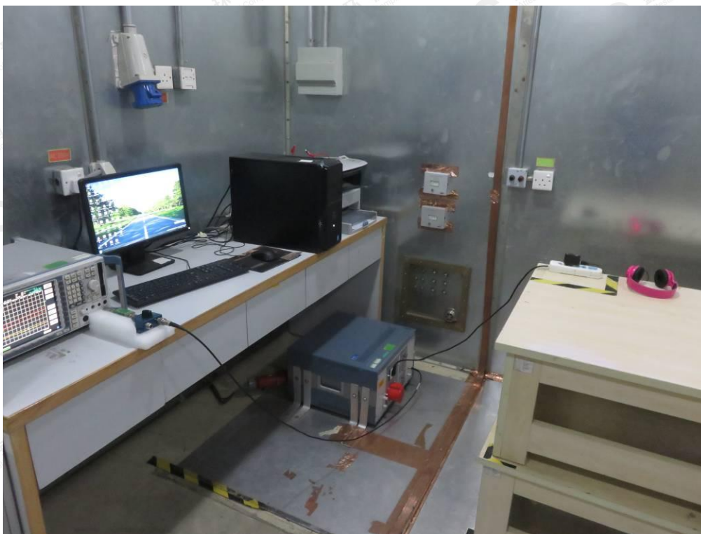
FCC RADIATED EMISSION TEST SETUP
