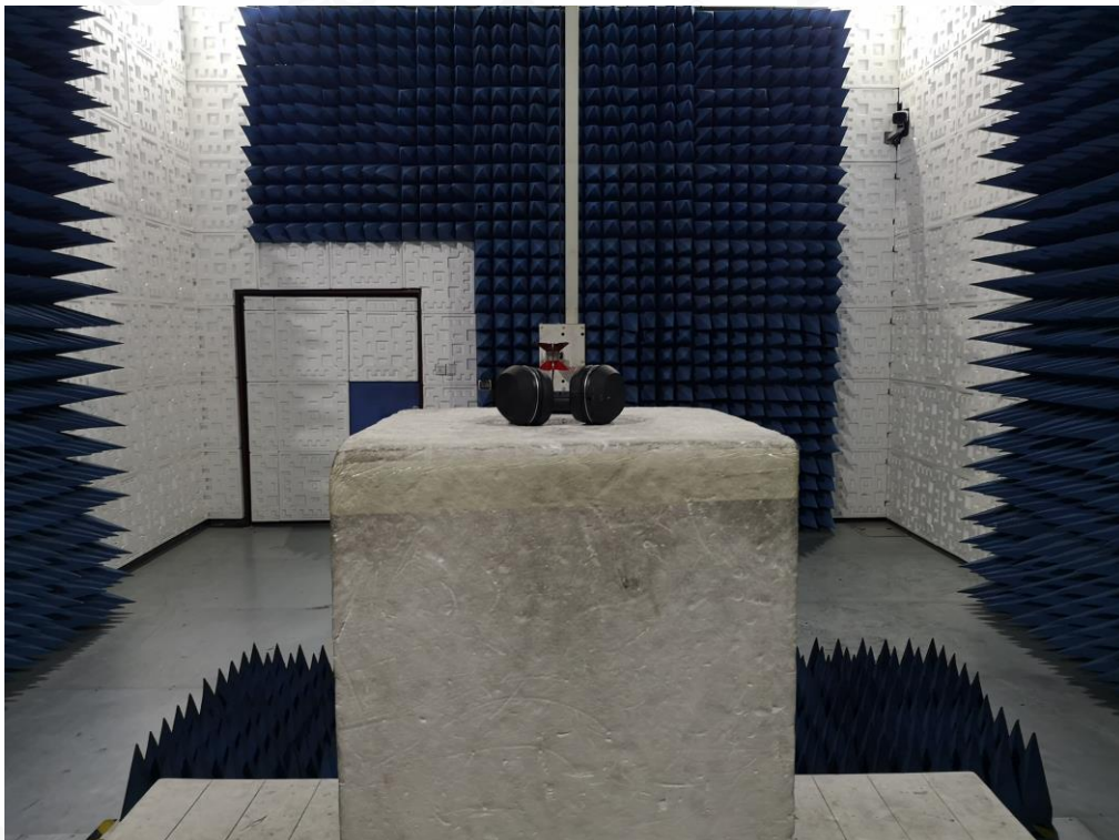
RADIATED EMISSION TEST SETUP ABOVE 1GHZ
