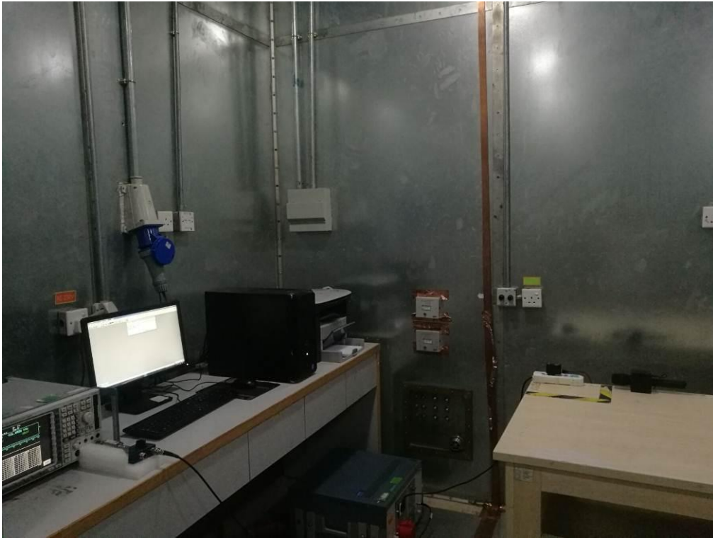
FCC RADIATED EMISSION TEST SETUP
