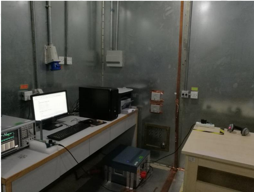
FCC RADIATED EMISSION TEST SETUP
