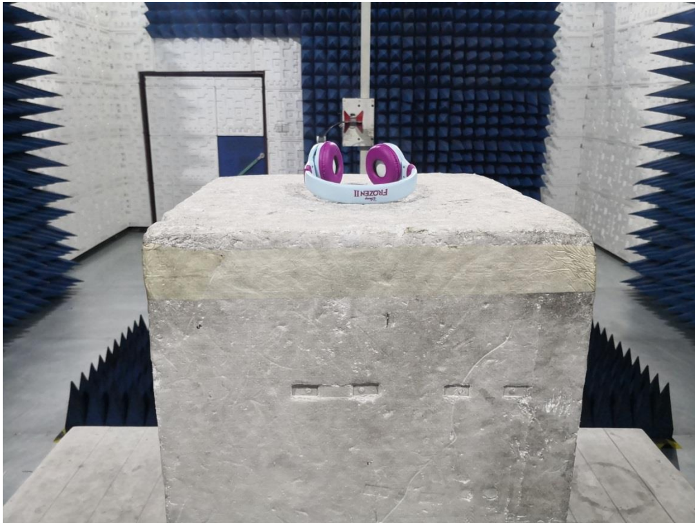
RADIATED EMISSION TEST SETUP ABOVE 1GHz
