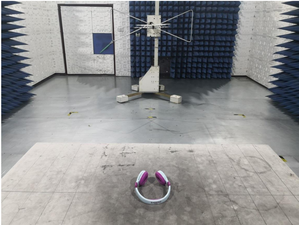
RADIATED EMISSION TEST SETUP ABOVE 1GHz
