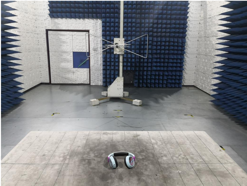
RADIATED EMISSION TEST SETUP ABOVE 1GHZ
