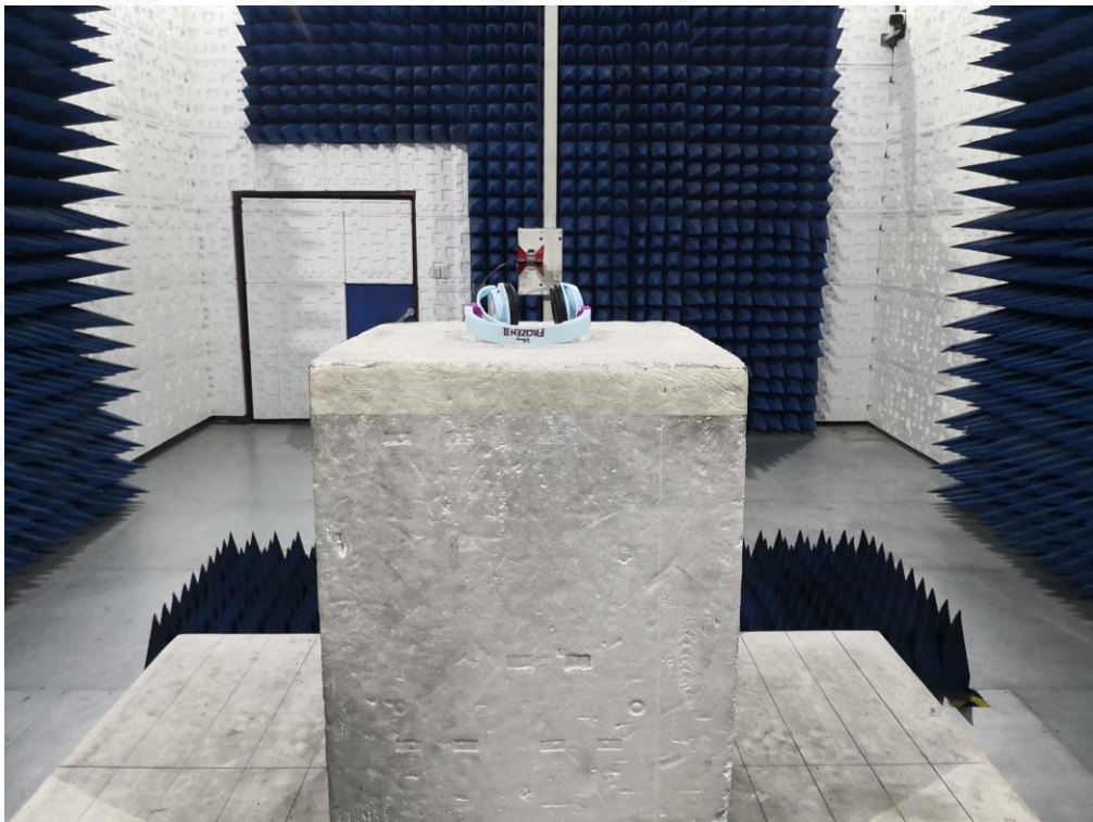
RADIATED EMISSION TEST SETUP ABOVE 1GHZ
