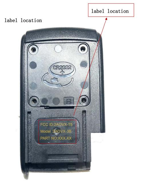
NOTE: The battery is not installed in the product when the product is sold to the customer. It must be installed by the customer themselves. Then customer will see the label when install battery.
