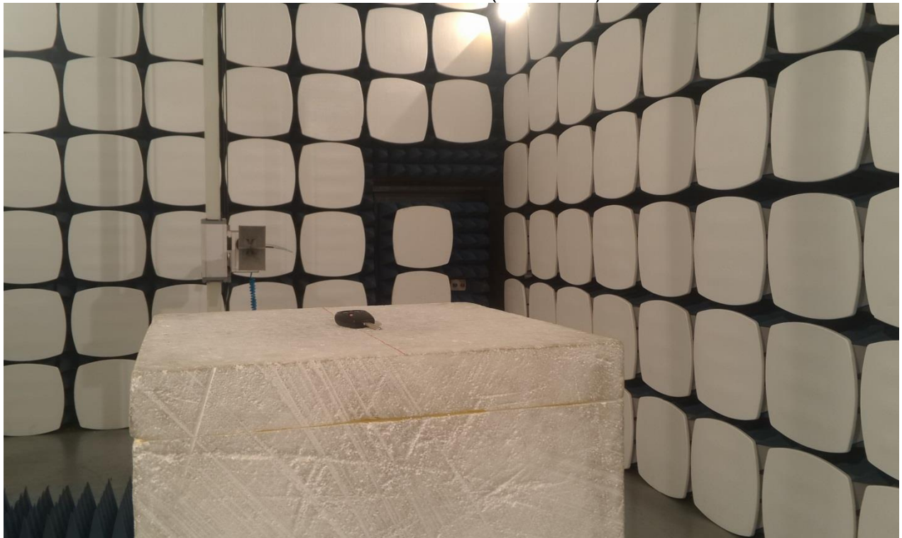
Radiated Emission(above 1G)
