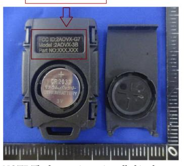
NOTE: The battery is not installed in the product when the product is sold to the customer. It must be installed by the customer themselves. Then customer will see the label when install battery.
