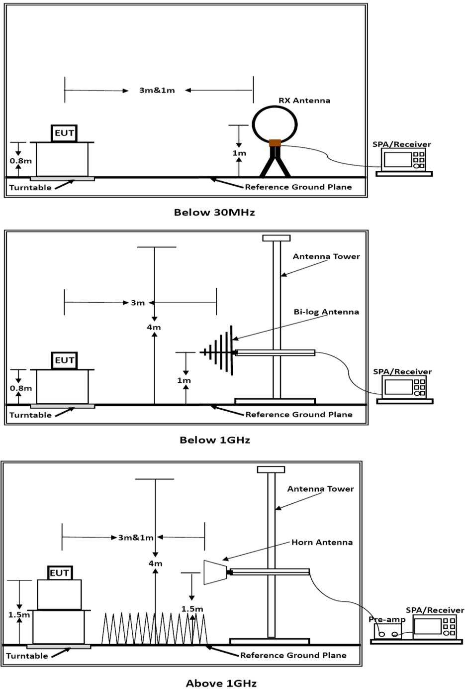
Above 10 GHz shall be extrapolated to the specified distance using an extrapolation factor of 20 dB/decade from 3m to 1.5m.
