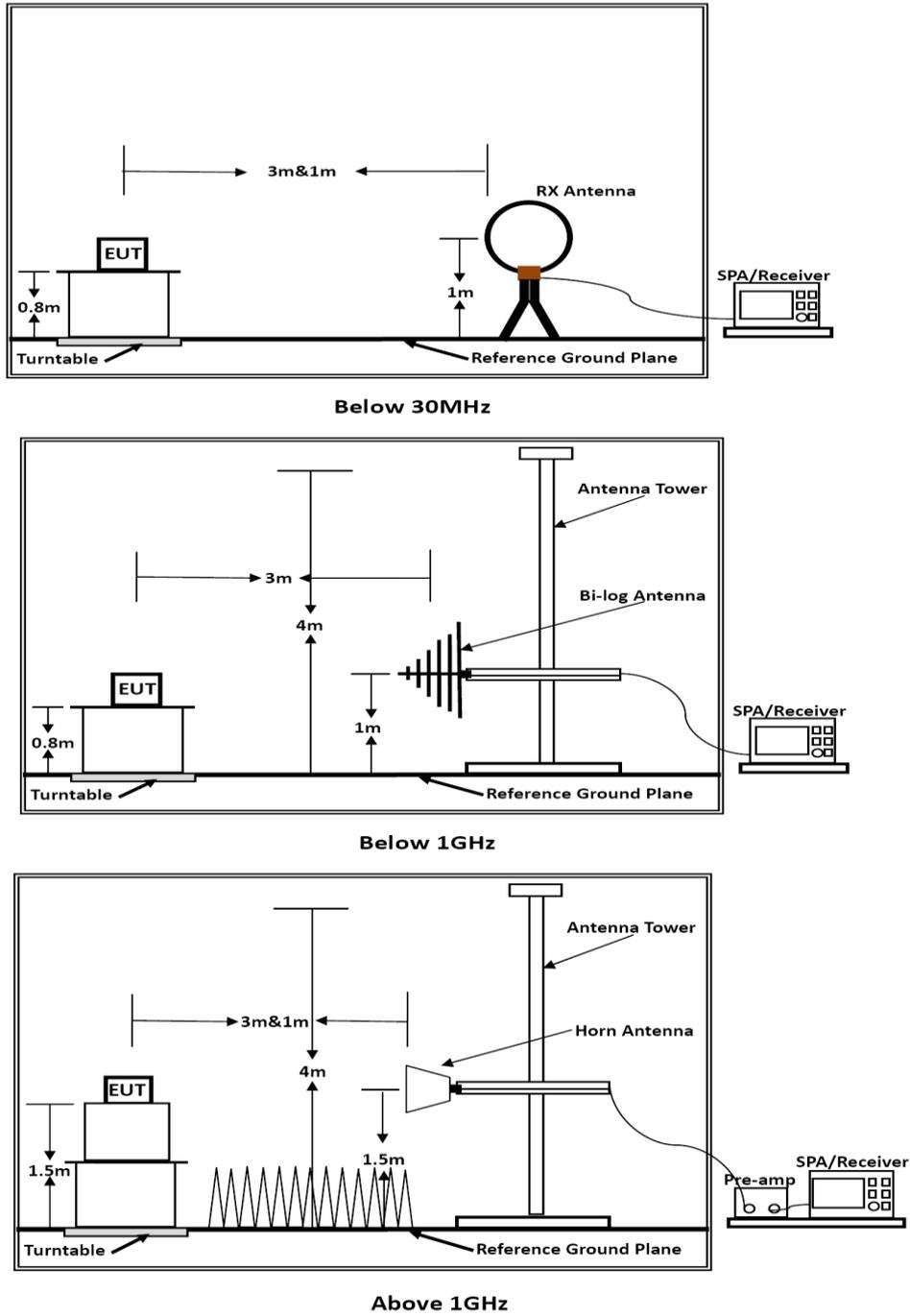
Above 10 GHz shall be extrapolated to the specified distance using an extrapolation factor of 20 dB/decade from 3m to 1.5m.
