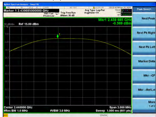
GFSK (BLE 1Mbps) MIDDLE CHANNEL
