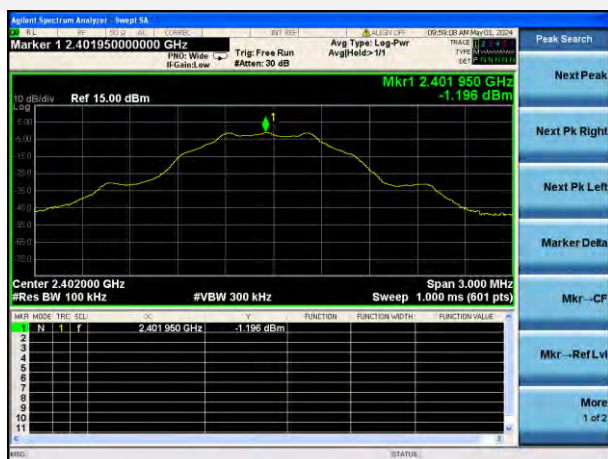
GFSK (BLE 1Mbps) LOW CHANNEL, CARRIER LEVEL
