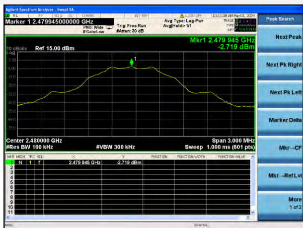
GFSK (BLE 1Mbps) HIGH CHANNEL, CARRIER LEVEL
