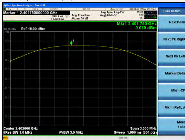
GFSK (BLE 1Mbps) LOW CHANNEL
