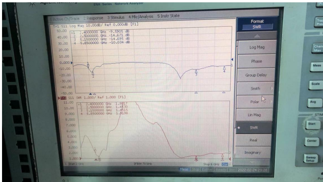
A antenna: dual-band WIFI antenna L=100mm VSWR
