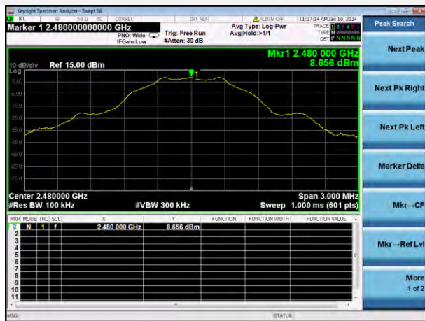
GFSK (BLE 1Mbps) HIGH CHANNEL, CARRIER LEVEL
