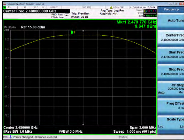
GFSK (BLE 1Mbps) HIGH CHANNEL
