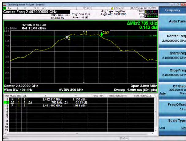
GFSK (BLE 1Mbps) LOW CHANNEL
