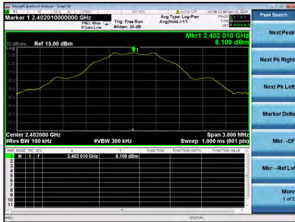
GFSK (BLE 1Mbps) LOW CHANNEL, CARRIER LEVEL
