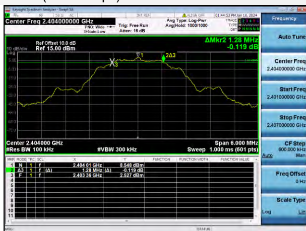
GFSK (BLE 2Mbps) LOW CHANNEL
