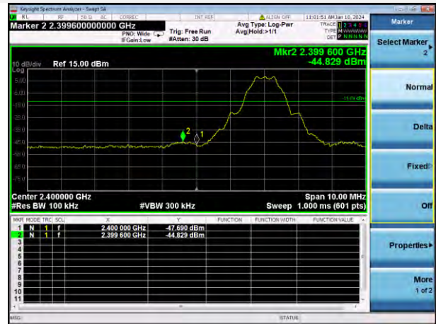
GFSK (BLE 1Mbps) HIGH CHANNEL, BAND EDGE
