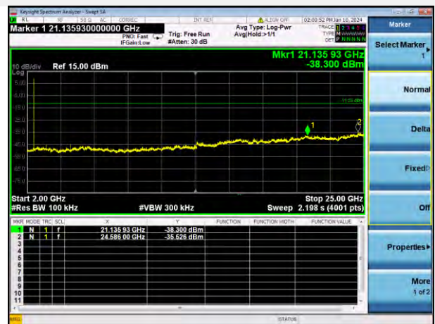
GFSK (BLE 2Mbps) HIGH CHANNEL, SPURIOUS 2 GHz ~ 25 GHz
