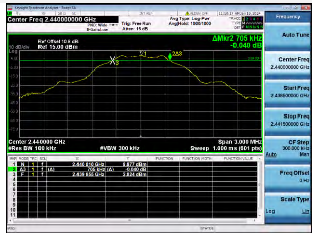
GFSK (BLE 1Mbps) MIDDLE CHANNEL
