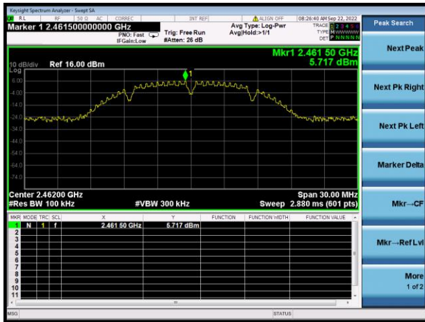
802.11b HIGH CHANNEL, CARRIER LEVEL
