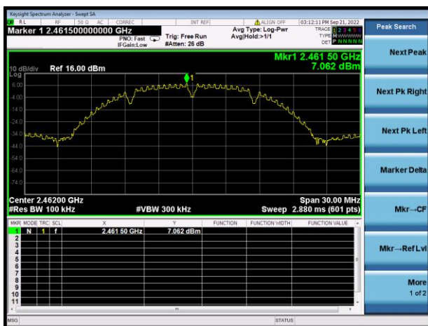
802.11b HIGH CHANNEL, CARRIER LEVEL
