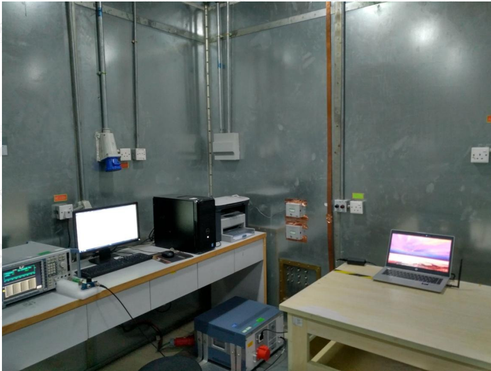
FCC RADIATED EMISSION TEST SETUP BELOW 1GHZ
