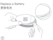
Please face to QR code side, and up lift open the back cover from silicone ring of the lower right corner.
