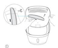
Install a filter to the back of water plate, and put the water plate back to water
