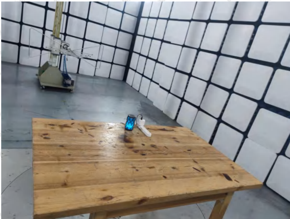
Photo of Radiation Emission Test
