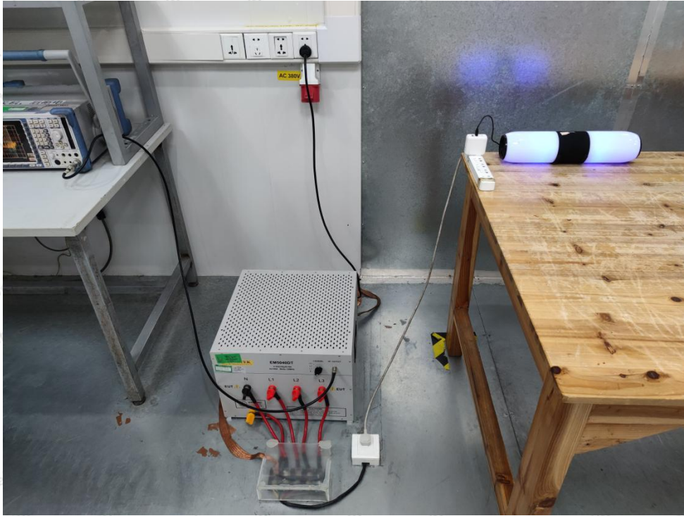
Photo of Conducted Emission Measurement
