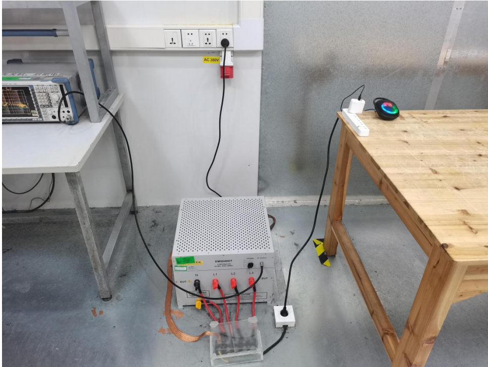
Photo of Conducted Emission Measurement
