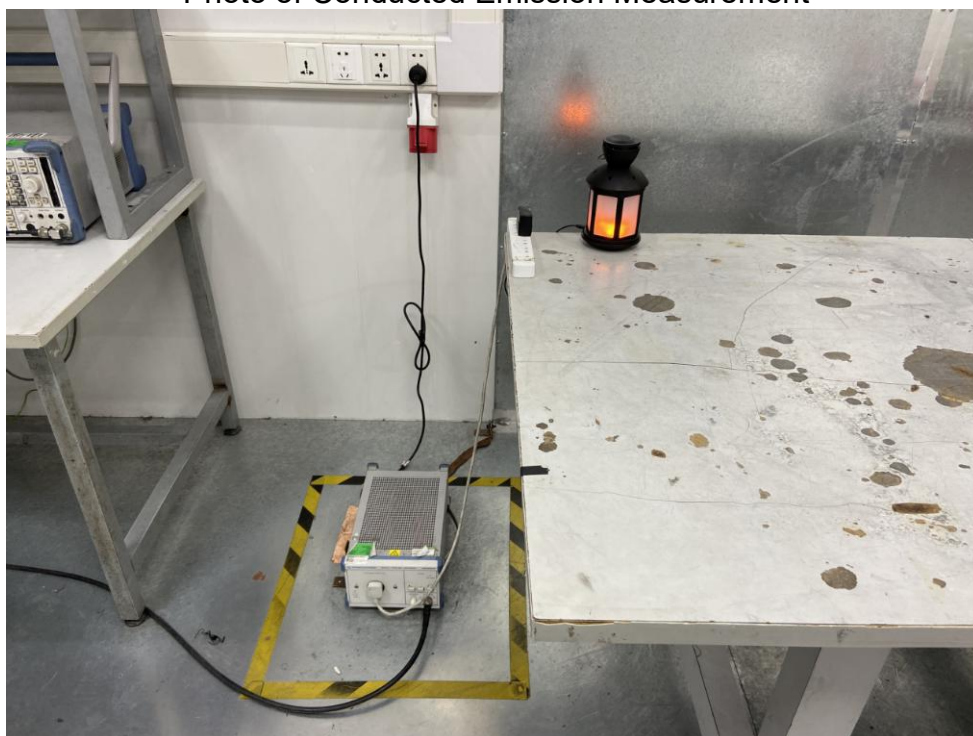
FCC ID: 2AOV6SP-228 Photo of Conducted Emission Measurement
