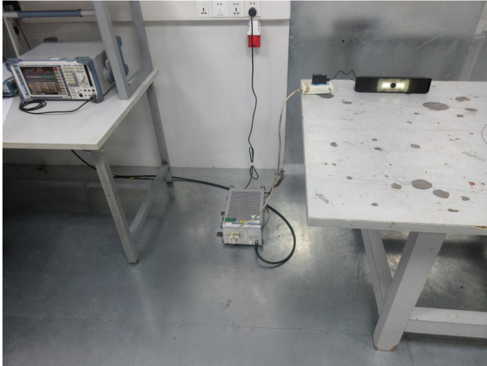
Photo of Conducted Emission Measurement
