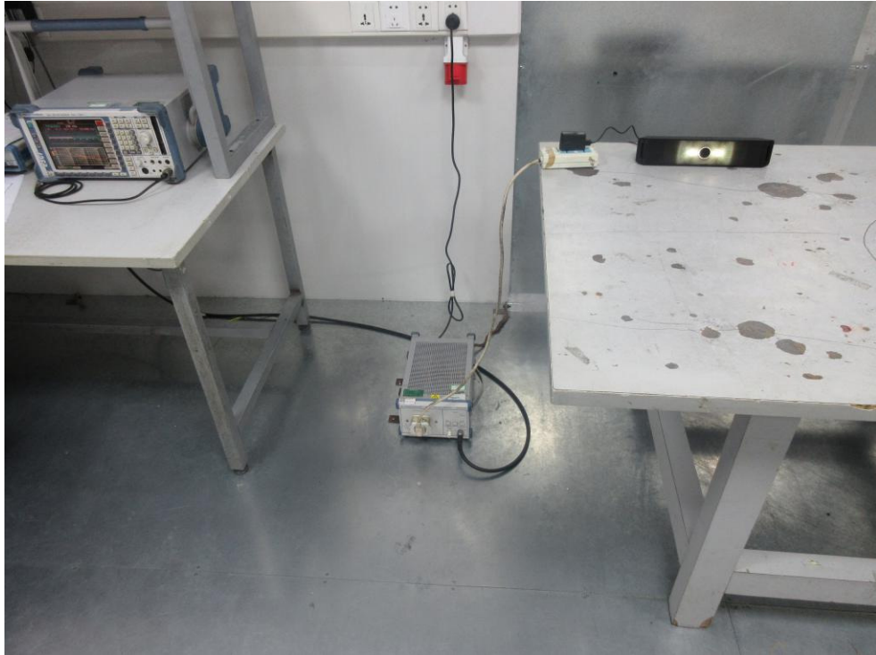
Photo of Conducted Emission Measurement
