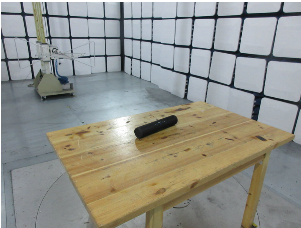
Photo of Radiation Emission Test
