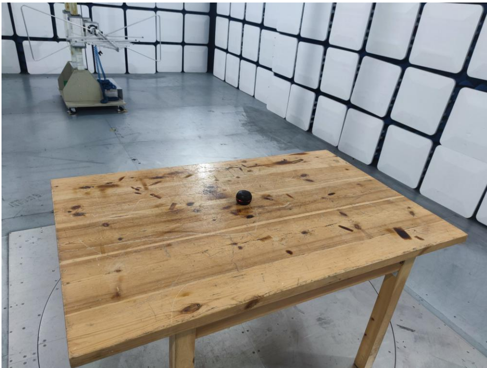
Photo of Radiation Emission Test
