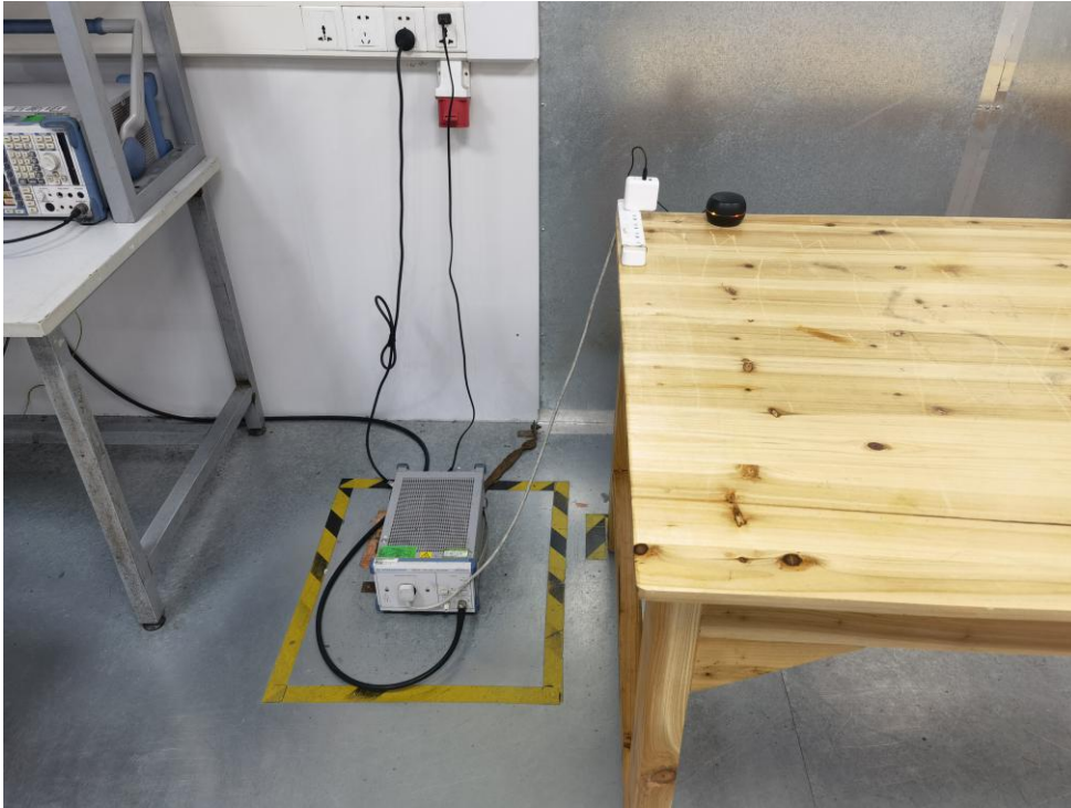
Photo of Conducted Emission Measurement
