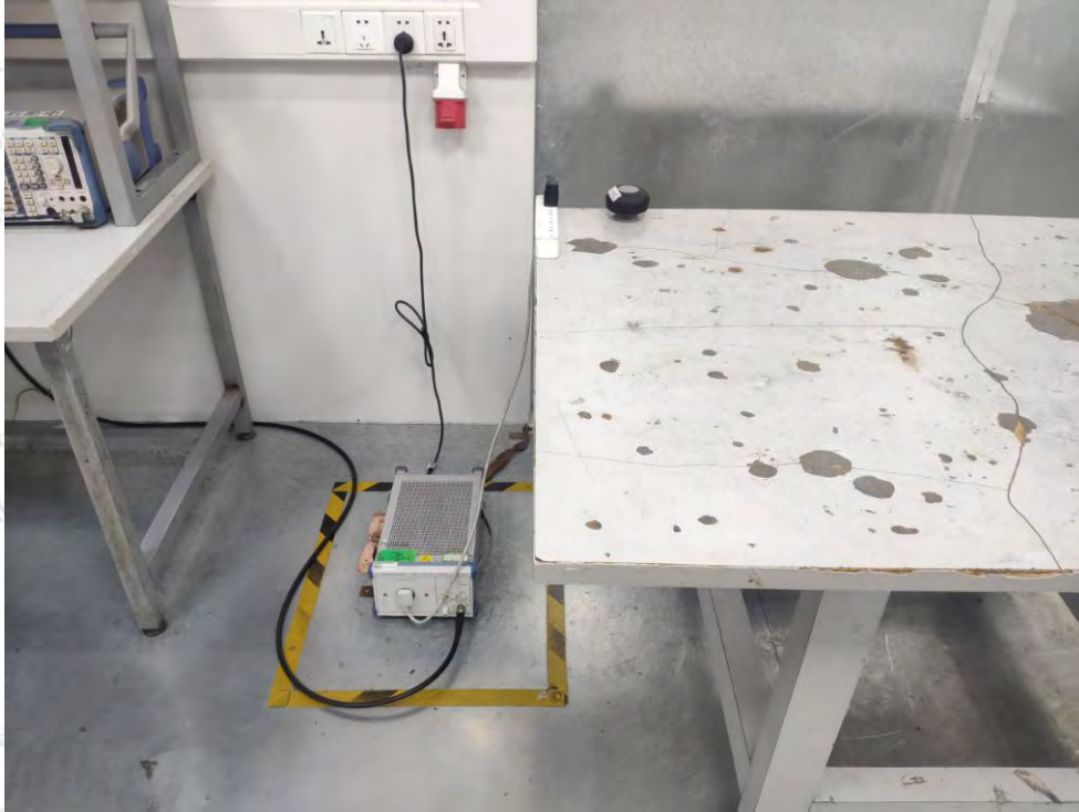
Photo of Power Line Conducted Emission Test
