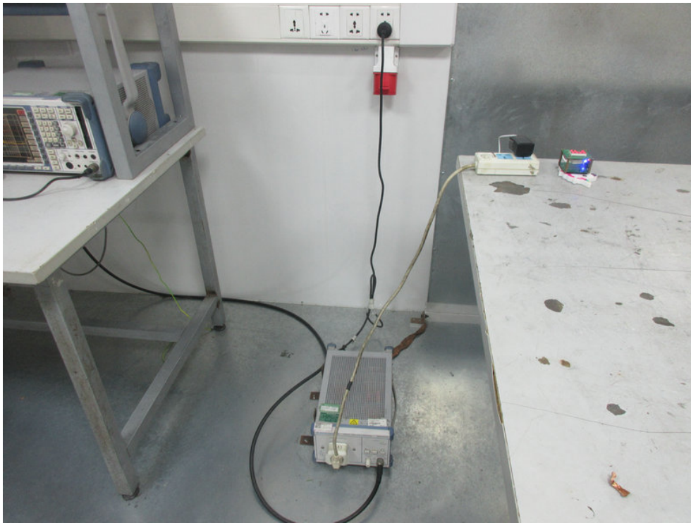
Photo of Conducted Emission Measurement
