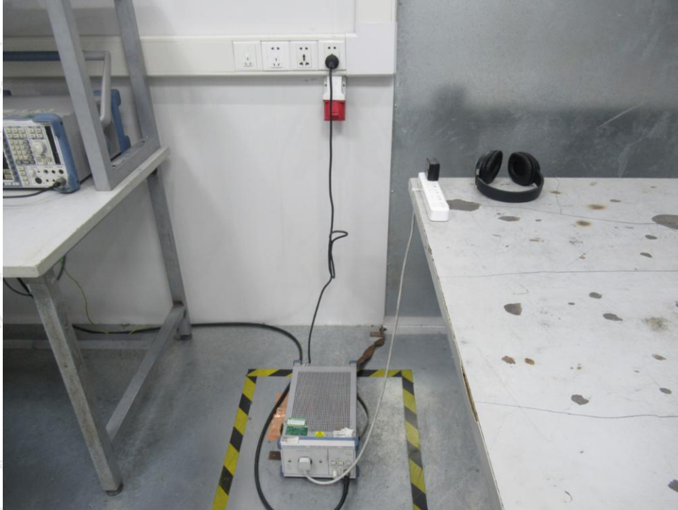
Photo of Conducted Emission Measurement
