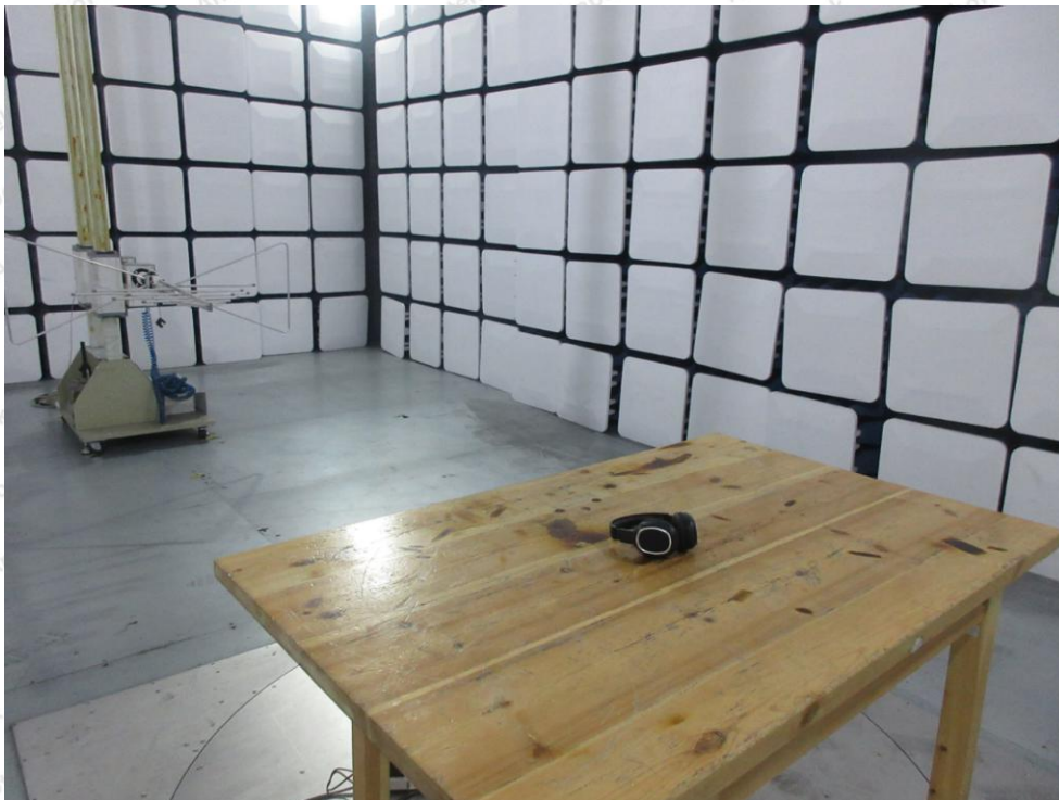
Photo of Radiation Emission Test
