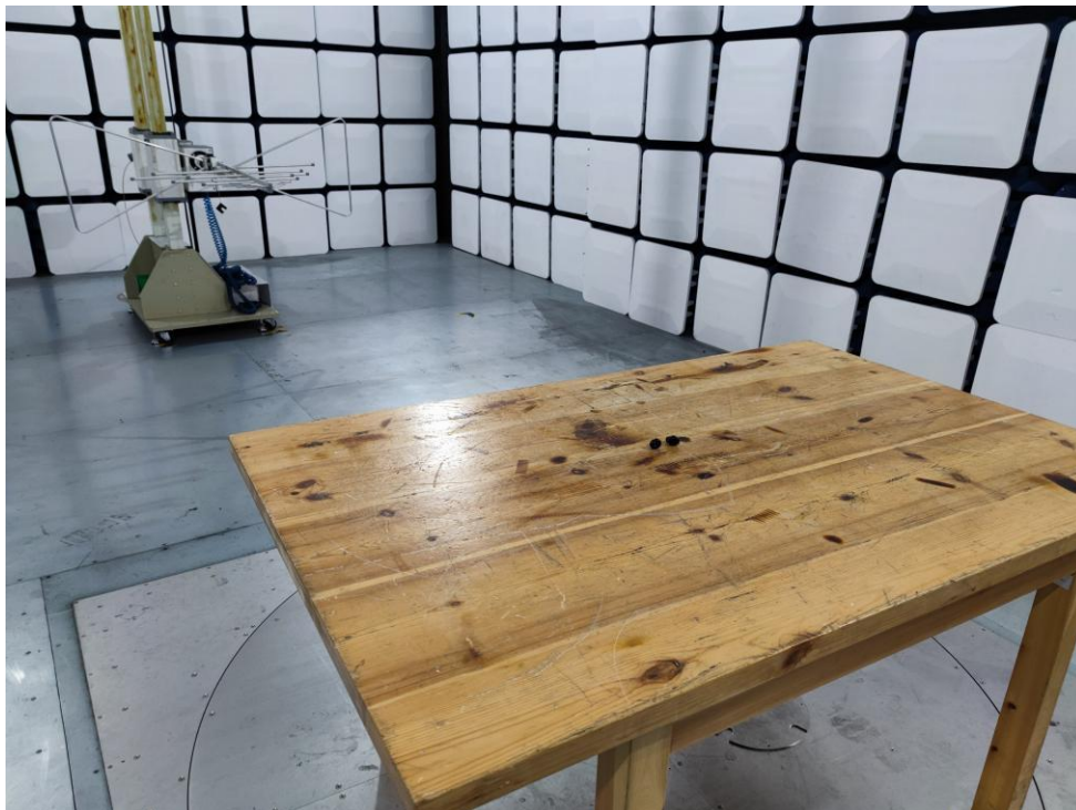
Photo of Radiation Emission Test
