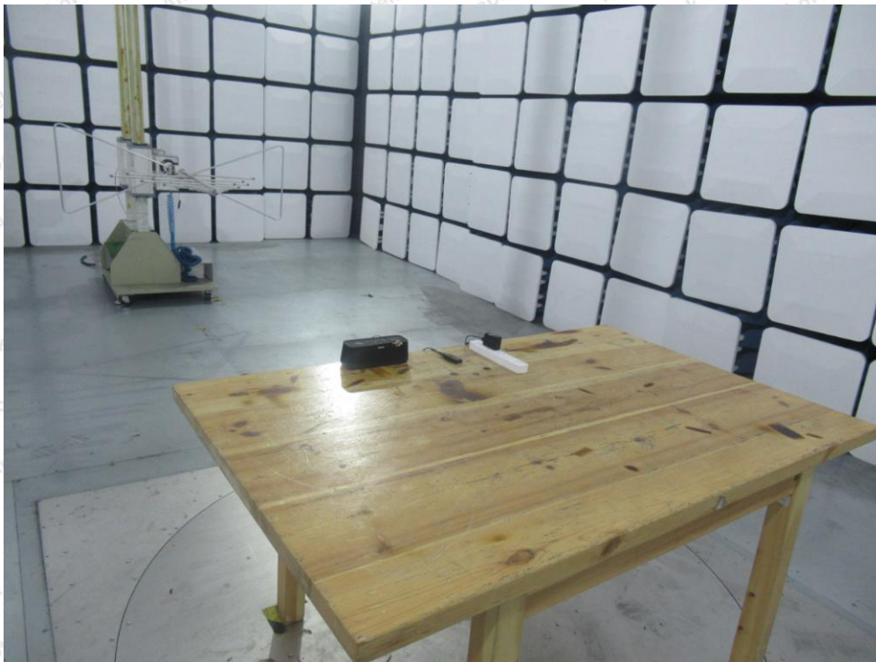
Photo of Radiation Emission Test
