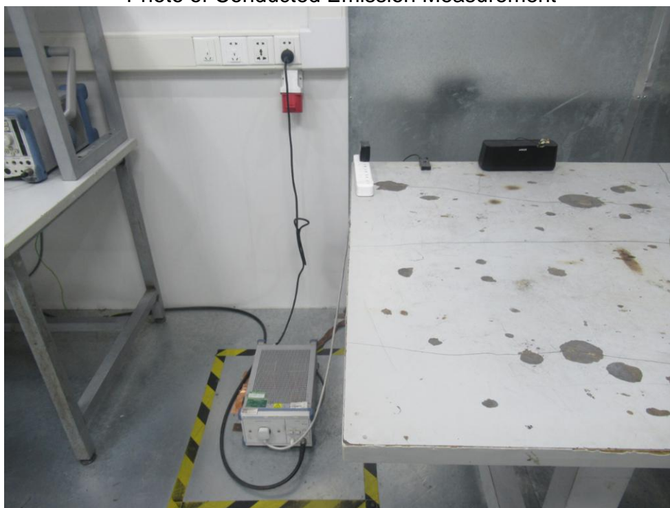
FCC ID: 2AOV6-BT001 Photo of Conducted Emission Measurement
