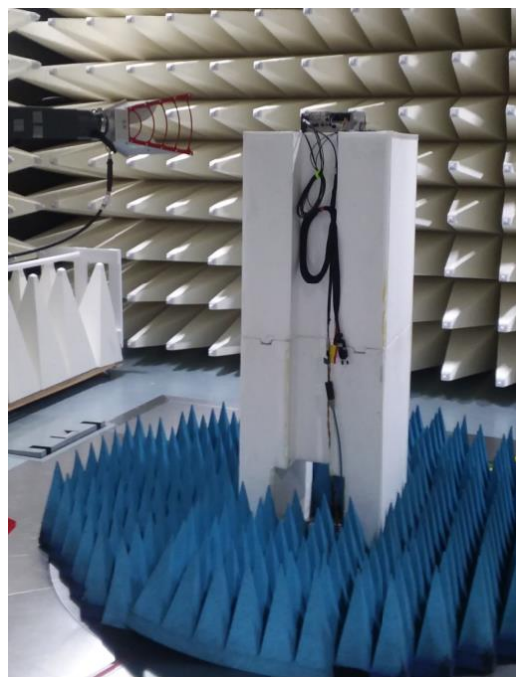
Figure D4: Radiated Emission Setup 2
